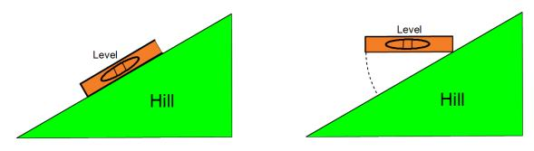
While holding the level/bottle still in this position, measure the distance between the end of the level and the ground using the ruler, as shown in the image below.
