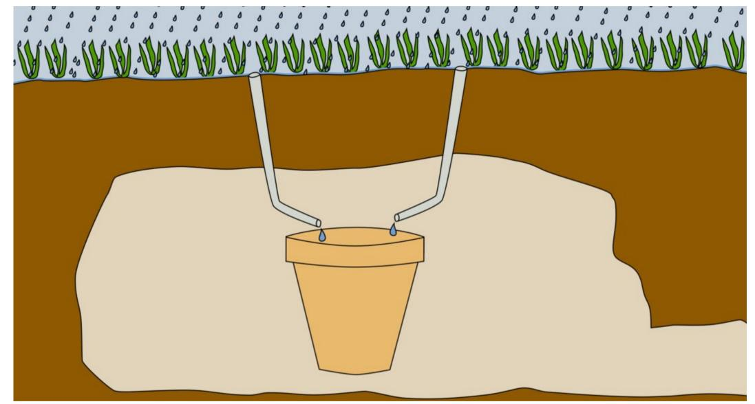
The installation of running water at their home was quite another thing. The first attempt was with straws connected to the surface. But the flow was too weak and during heavy rains the mud rose obstructing the mouth of the pipes.
