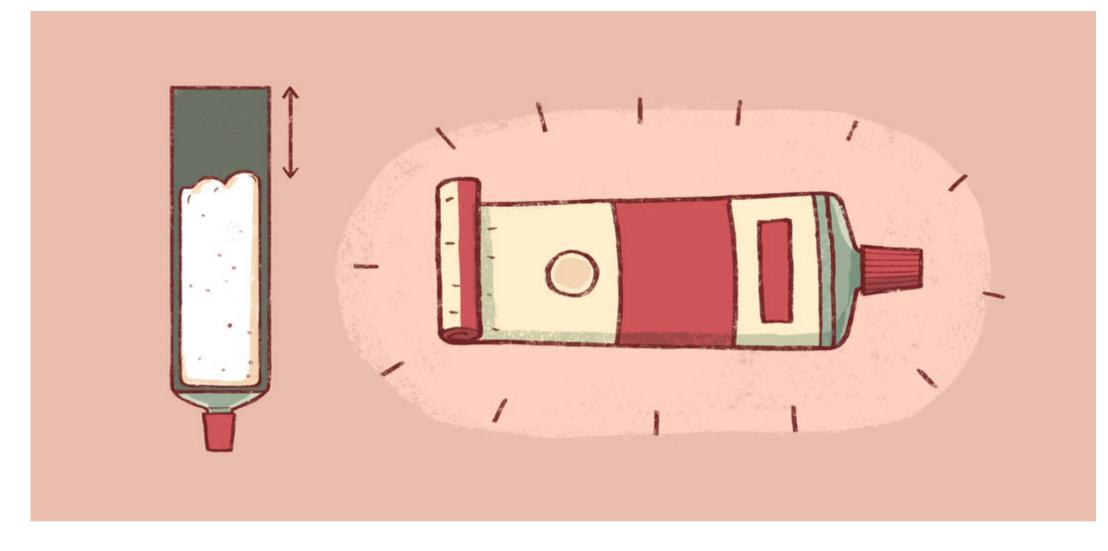
From a nozzle at the bottom of the container, the toothpaste is let into each of these tubes as they move along the conveyor belt. But the paste is not filled all the way to the brim. About half an inch is left so that it can be sealed.
