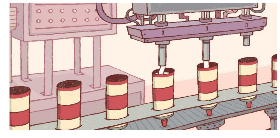
Today, toothpaste tubes are filled using machines. All the empty tubes are lined up on a conveyer belt with their caps downwards and the unsealed end pointing up. A big container filled with toothpaste is fixed above the conveyor belt.
