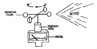
Fig 29: A cup anemometer
