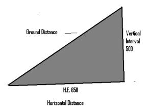
Figure 20: Gradient of a slope
