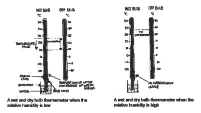
Fig 23: A wet and dry bulb thermometer
