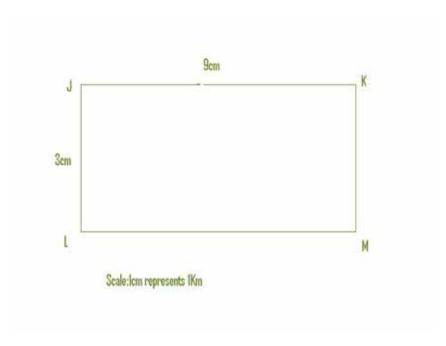
To calculate the area of JKLM, calculate the actual ground distance for JM and JL. If we use a scale of 1cm representing 1 km we get the following:
