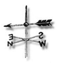
The wind vane is an instrument made up of horizontal arms pointing in the four main compass directions. At the centre of the arms is a freely rotating vertical shaft, which has a horizontal arrow on top. When wind blows, the arrow moves until it points at the direction from which the wind is blowing.
