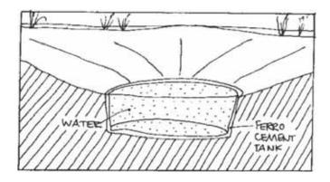
Fig 6: Ground catchment system.
