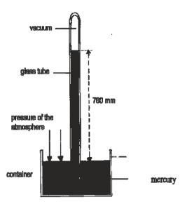
Fig 31: A mercury barometer
