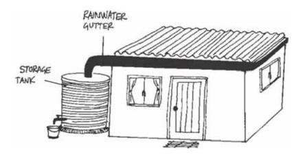
Fig 5: Roof catchment system
