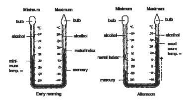
Fig 9: A minimum and maximum thermometer
