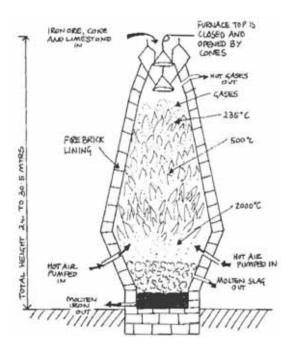
Figure 3: A Blast Furnace
