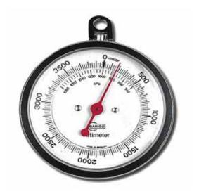
Fig 33: An altimeter Downloaded from  $\underline{http://geometrytech3.wikispaces.com/file} \ on \ 23/5/11$
