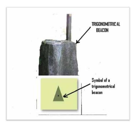
**Figure 37: A trigonometrical beacon adapted from** <u>flickr.com/photos/kinetawherlock/3759010364/</u> on 7/12/10
