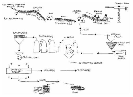
Figure 9: Stages in the processing of sugar
