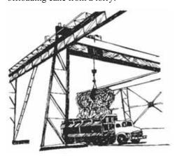
Figure 8: A crane unloading cane from a lorry
