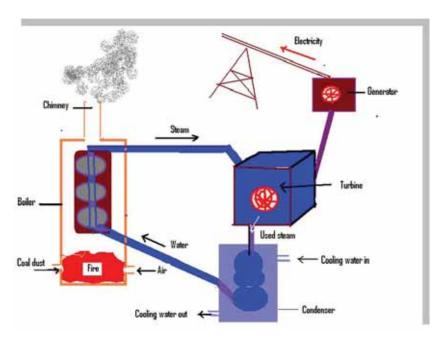
Figure 17: The process of generating power from coal. (Adapted from - jpgprojectmidori.com) on 12/03/10
