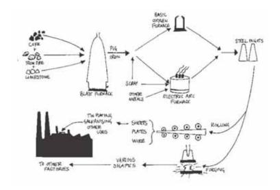
Figure 2: Integrated Process of producing iron and steel at Vanderbijl Integrated Steel Works
