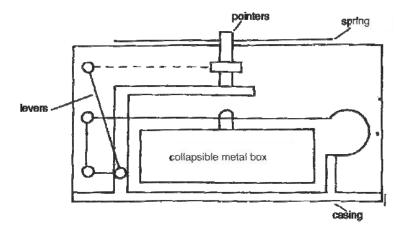
Fig 32: An aneroid barometer
