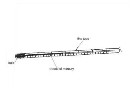
Fig 6: A simple mercury thermometer
