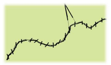
Measure each of these sections with a pair of dividers and write down each measurement. Add the length of each of the straight sections. Then use the linear scale to find out the actual distance on the land.
