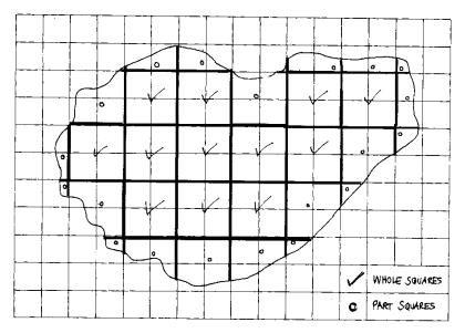
If you use a metric graph paper, one large square measures  $2 \times 2$  cm. If the scale of a map is 1 centimetre to 1/2 kilometre or 500 metres, each large square is equivalent to 1 square kilometre of land. If a scale of 1 centimetre to 1 kilometre is used, then each large square represents 4 square kilometres of land.
