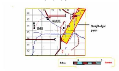
Keep on moving the paper along the curves or bends, each time making a mark on the edge of your paper where a new curve starts and ends until you reach the end of the line, in this case F.
