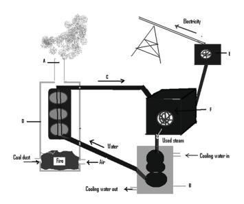
The process of generating power from coal (Adapted from -  $\underline{jpg}$  projectmidori.com ) on 12/03/10
