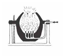
Figure 4: A Bessemer Converter Furnace
